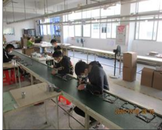
Photo of non-conformity NC-No local exhaust ventilation system for soldering area.JPG
